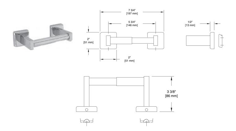
MATERIALS: Inner Wall Flange - 16 gauge type 304 stainless steel
