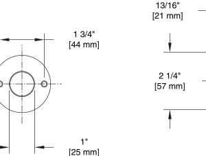
**MATERIALS:** 1" O.D. x .020 (25 gauge) seamless chrome plated brass. Flange material as listed under each model number.
