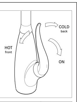
If the handle is installed on the left side hot water is obtained by moving the lever backward and cold water by moving it forward and water flow is turned on by moving the handle to the left.
