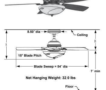
Fan must be attached to a securely anchored electrical junction box capable of withstanding a load of at least 50 lbs.
