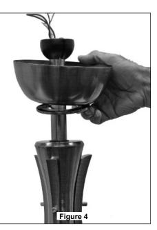
4. Re-assemble the Canopy Screw Cover, Canopy, and downrod hanger ball assembly. Reinstall the Hanger Ball (Figure 4) on the Downrod as follows. Position the Pin through the two holes in the Downrod and align the Hanger Ball so the Pin is captured in the groove in the top of the Hanger Ball. Pull the Hanger Ball up tight against the pin. Securely tighten the setscrew in the Hanger Ball. A loose setscrew could create fan wobble.
