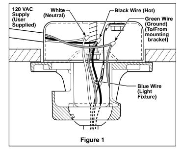
**5.** After connections have been made, turn leads upward and carefully push leads into the outlet box, with the white and green leads to one side of the box and the black and blue leads towards the other side.
