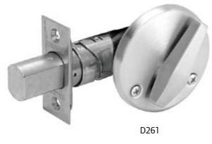
Deadbolt thrown or retracted by turn unit only. Occupancy indicator on outside (reads either "in use" or "vacant" with color coding). Bolt automatically deadlocks when fully thrown. Emergency key supplied.
