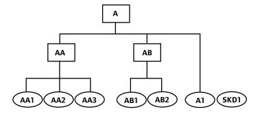
When locks are required which are not operated by ANY master keys or other change keys in the system, they are referred to as "single keyed" and given symbols **SKD1**, **SKD2**, etc.
