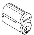
With Best® style capping, each pin chamber is sealed with its own individual cap.
