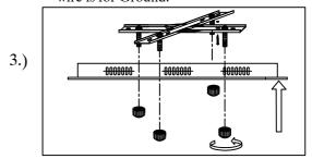
Step.3: Screw finials (D) onto mounting bracket (A) until canopy is flush with ceiling.
