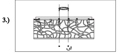
Step.3: Screw finials (D) onto mounting bracket (A) until canopy is flush with ceiling..
