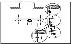
Step.1: Remove mounting bracket (A) and install to electrical box. Mark where anchors meet ceiling, remove mounting bracket from ceiling, and then drill holes using 3/16" drill bit where marked (B). Install mounting bracket and attach anchors to secure bracket at ends.
