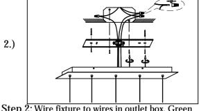
Step.2: Wire fixture to wires in outlet box. Green
