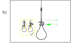
Step.3: Install G9 bulb (D) provided. Gently turn glass (E) onto socket to secure.
