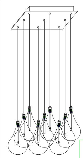
WARNING: Wires need to be connected to transformer found in canopy and should not be connected directly to power source or a short may occur
