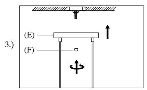
Step 3: Install fixture to bracket using finial (F) to secure.
