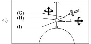
Step4: Twist the plastic screws(G) with a screwdriver, use the six angle wrench to loosen the inner six corner screws(H), and twist the cylindrical iron(I) parts.
