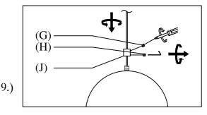
Step9: To tighten cylindrical iron(J) parts, first lock the inner hexagonal screw(H) with an inner hexagonal wrench, and then lock the plastic screw(G) with a screwdriver.
