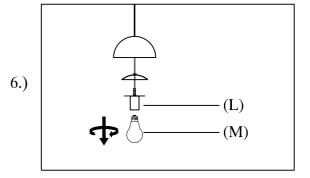
Step6: Turn the bulb out of the socket.
