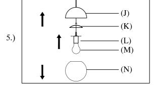
Step5:Open the semicircle lampshade(J), twist the nut and take out the Flange(K) and the lamp socket(L) and Glass(N).
