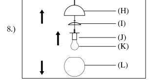
Step8: Tilt the lamp socket(J) into the Glass(L). Place the Glass(L) flat, cover the Flange(I), tighten the nut and cover the upper Semicircular lampshade(H).
