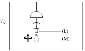
Step7: Twist the new bulb(M) into the lamp socket(L).
