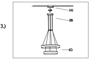
Step 3: Adjust wire length to desired hanging height. Install Canopy (B) to Bracket (A) and tighten screws at the ends of canopy to secure.
