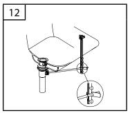
Place one end of spring clip on end of ball rod. Insert rod across and through hole in lift rod strap. Secure other end.
