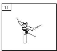
Thread locknut from underside of sink until rubber washer seats securely inside opening of sink. Tighten locknut. Wipe off excess putty. If model has plastic wing nut, tighten securely by hand. If nut is brass, tighten with a wrench.
