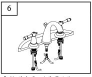
Position the bodies as in the illustration to install quick-connect on hot and cold inlets. Carefully bend the hoses to fit available space.
