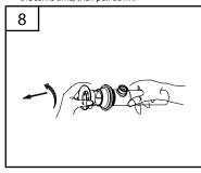
Remove flange from pop-up main body. Leave large black washer (not included with plastic pop-up) and nut on drain body.
