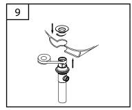
Add PTFE pipe tape to the threads on the drain body. Add Plumbers Putty to the bottom of flange per manufacturer's directions. Insert threaded end of drain body up through drain hole and attach flange to body with ball rod pointing to the rear of sink. Tighten the flange.
