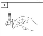
Locate water supply inlet and shut off water supply valve. These are usually found under the sink or near the water heater. Remove old faucet. Clean and dry sink surface area where new faucet will be mounted.
