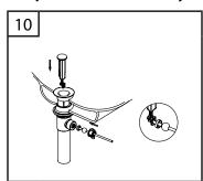
Unscrew the nut from the pop-up body and take off the spring clip from the ball rod (Please note: The white packing ring must remain on the ball rod). Place the nut on the ball rod. Insert the ball rod into the side hole of drain, slide the nut on and tighten securely.
