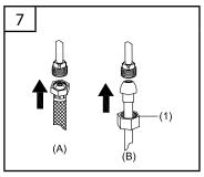
Connect water supply lines. (A) Use 1/2" IPS faucet supply lines or use coupling nuts (not supplied) with ball-nose risers (not included).
