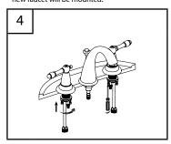
Insert the valve body labeled hot supply on the left (hot)side. Hold the body in the proper position. Assemble metal washer, mounting nut and screw onto body on underside of sink. Firmly tighten the lock screws to the metal washer. Repeat the same procedure for the right (cold) side.
