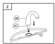
Be sure that flange (2A) is placed on the bottom of spout body (2B). Insert spout shank (2C) through the center hole of sink.
