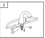
From underside of sink, place rubber washer and metal washer (3A) onto spout shank (3B) and tighten mounting nut (3C).
