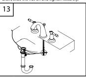
Insert bottom of lift rod into hole at top of pop-up strap. Tighten thumb screw.
