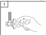
Locate water supply inlet and shut off water supply valve. These are usually found under the sink or near the water heater. Remove old faucet. Clean and dry sink surface area where new faucet will be mounted.
