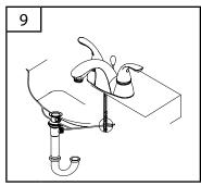
Insert bottom of lift rod into hole at top of pop-up strap. Tighten with thumb screw.
