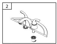
Place new faucet through holes in top of sink. From underside, slide washers onto threaded rods. Secure with washer and nuts.
