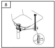
Place one end of spring clip on end of ball rod. Insert rod across and through hole in lift rod strap. Secure other end.
