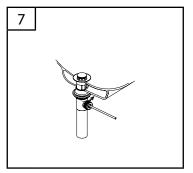
Thread locknut from underside of sink until rubber washer seats securely inside opening of sink. Tighten locknut. Wipe off excess putty. If model has plastic wing nut, tighten securely. If nut is brass, tighten with a wrench
