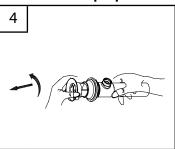
Remove flange from pop-up main body. Leave large black washer (not included with plastic pop-ups) and nut on drain body.
