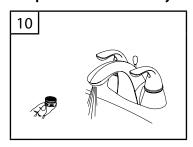
Important: After installation is completed, remove aerator. Turn on water supply and allow both hot and cold water to run for at least one minute each. While water is runner, check for leaks. Replace aerator. Tighten nuts slightly to stop minor leaks. If problems persist, refer to troubleshooting chart.
