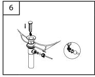
Unscrew the nut from the pop-up body and take off the spring clip from the ball rod (Please note: The white packing ring must remain on the ball rod) Place the nut on the ball rod (Insert the ball rod onto the side hole of drain, slide the nut on and tighten securely.
