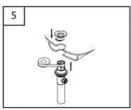
Add PTFE pipe tape to the threads on the drain body. Add Plumbers Putty to bottom of flange per manufacturers directions. Insert threaded end of drain body up through drain hole and attach flange to body with ball rod pointing to the rear of the sink. Tighten the flange.
