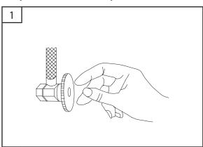
Locate water supply inlet and shut off water supply valve. Remove old shower head. Clean and dry surface area where new shower head will be mounted.
