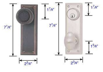
Non-Keyed Passage (8104) Privacy (8204) Dummy (8054) Keyed 3 %" C-to-C Single Cylinder (8080) Double Cylinder (8081) Dummy (8085)
