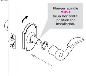
**Step 2.** Tighten lever set screw after placing lever on stem.
