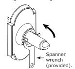
**Step 1.** Secure inside rosette to door by threading it clockwise on to stem.
