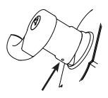
**Step 2.** Rotate key counterclockwise 90° while pressing wire into hole.
