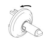
**Step 1.** Secure inside rosette to door by threading it clockwise on to stem.
