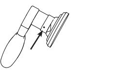
**Step 2.** Rotate key counterclockwise 90° while pressing wire into hole.
