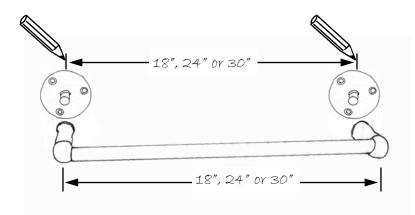
Use a screw driver to install three Screw Anchors into the wall for each mounting plate. Install mounting plates on top of the Screw Anchors. Attach with the sheet metal screws provided.
