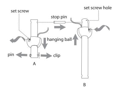
**Tip:**To prepare for threading electrical wires through downrod, apply small piece of electrical tape to the ends of the electrical wires--this will keep the wires together when threading them through the downrod.
