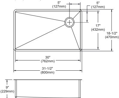
Installation Profile of ECTRU Models
