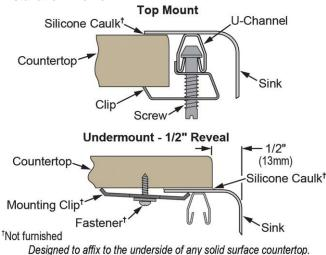
Designed to anix to the underside of any solid surface counte
