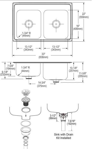
Sink with Drain Kit Installed
