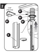
For countertop thicknesses less than 1/16" thick use the rubber gasket (B1) and mounting flange (B2), for all other installations use the rubber gasket (B1) and metal washer (B3).
