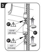
Install the check valve (C1) to the outlet hose with a rubber washer (C2)
