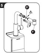
Tighten the shower (F) to the hose interposing the gasket (D3) and confirm the hose can slide smoothly through the passage hole.
