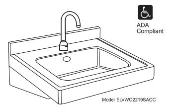
state, has adjustable sensorrange of 7/8" (22mm) to 6-3/4" (171mm), shut-off delay preset at 1 second and field adjustable to 2 seconds (to prevent sink overflow).
