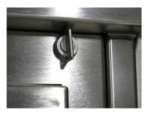
Cycle water and soap buttons to verify proper operation of water switch and soap pump.
