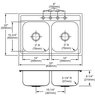
**Hole Drilling Configurations**
