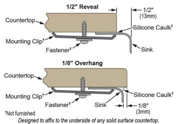
PART:\_\_\_\_\_QTY: \_\_\_\_\_ PROJECT:\_\_\_\_\_ CONTACT:\_\_\_\_\_ DATE:\_\_\_\_\_ NOTES:\_\_\_\_\_ Harmony<sup>™</sup> (Lustertone®) Stainless Steel Single Bowl Undermount Perfect Drain Sink Model(s) ELUH1716PD
