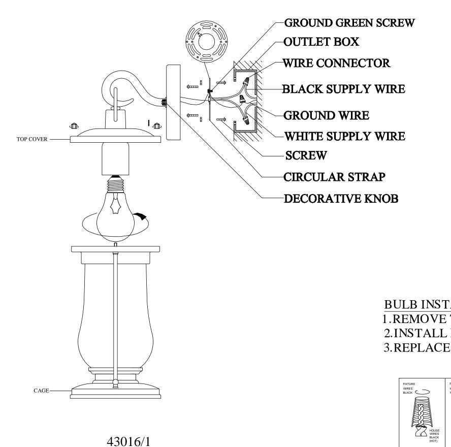
BULB INSTALLATION OR REPLACEMENT 1.REMOVE THE CAGE FROM THE TOP COVER DIRECTLY. 2.INSTALL BULB. 3. REPLACE THE CAGE TO THE TOP COVER DIRECTLY.
