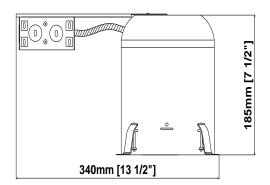
**HOUSING:** Pre-wired.042" aluminum housing adjusts up to 1 3/4" ceiling thickness. Trim is secured with torsion wing springs/standard coil springs. NONIC rated housing may have direct contact with insulation.
