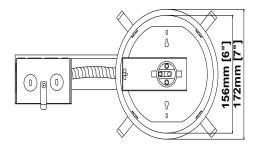
**MOUNTING FRAME:** 4High tension remodeling clips designed to secure the housing to an existing sheet rock ceiling
