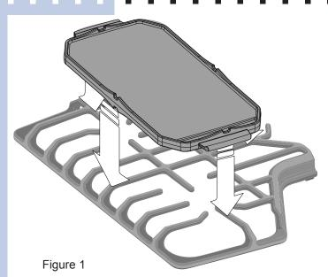
The griddle is intended for direct food cooking and can be used on both sides. **Do not** use pans or other cookware on the griddle. Doing so could damage the finish. With the grate in position over the burner, set the griddle on top of the grate positioning the notches in the griddle over the grate fingers (refer to figure 1 for optimal positioning).
