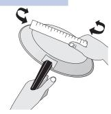
Pans should have flat bottoms. Check for flatness by rotating a ruler across the bottom. There should be no gaps between the pan and ruler.
