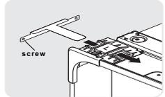
To install using Top Mount Cabinet Clips: Depending on the depth of cabinet, the Top Mount Clip have a break off point that can be removed if necessary.
