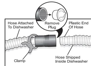
3. Take the plastic side of the drain hose and insert it into the hose that is already attached to the dishwasher make sure hose ends are flush against each other. See image below.
