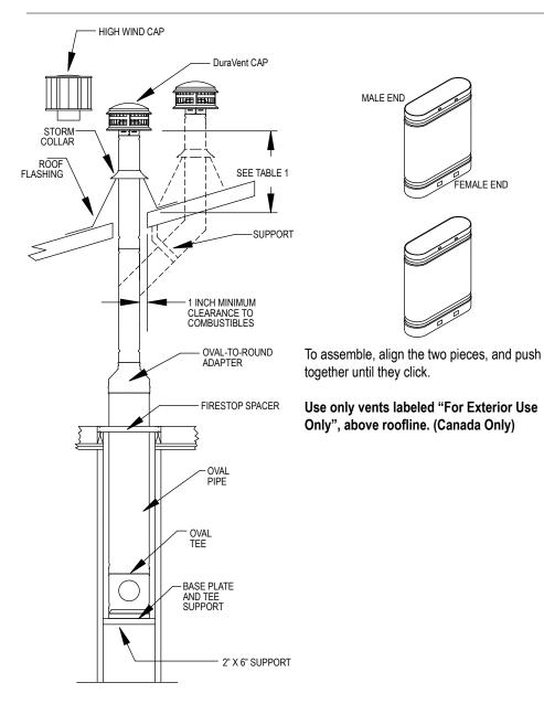
Diagram showing transition from 6" oval to round vent pipe, and optional offset. Note that offsets must be supported
