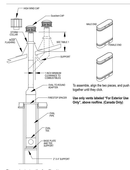
Diagram showing transition from 5" oval to round vent pipe, and optional offset. Note that offsets must be supported
