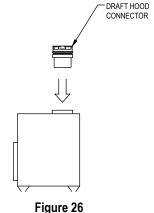
the appliance manufacturer for clarification. Place the appliance out in front of the fireplace area, as shown in *Figure 27*, and install the Draft Hood Connector, or other device in accordance with the appliance instructions. The Flex Pipe Coupling may be able to attach directly to the appliance.
