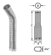
Use through damper and smoke shelf area. Use to connect from oval stove outlet to round DuraLiner. Use with DuraLiner ProMesh and ProFoil, where flex extends into clay liner, for zero-clearance applications. Built from 1-ply construction, .005" 304 stainless steel.
