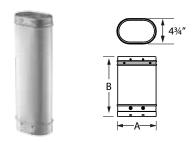
Use to reline masonry chimney with 0/0 clearance. Available in oval 6" and 8" diameters; 12", 24", 36", and 48" lengths. Factory-insulated. Built-in, pre-drilled fittings for riveting joints. 304 stainless steel inner and aluminized steel outer. Note: to calculate the installed length of 5", 6", and 8" DuraLiner pipe subtract 1  $\frac{1}{2}$ " from each joint overlap of liner pipe sections.
