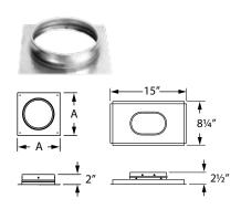
Use to connect stove to round or oval DuraLiner pipe. Oval stove connector is sized to convert round stove outlets to oval DuraLiner pipe.
