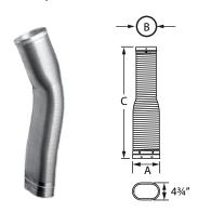
Use through damper and smoke shelf area. Use to connect from round stove outlet to oval DuraLiner. Use with DuraLiner ProMesh and ProFoil, where flex extends into clay liner, for zero clearance applications. Built from .016", 304 stainless steel, 4-ply construction.
