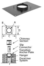
Use with Slip Connector and Hanger in chimney restoration to connect DuraLiner pipe to DuraTech, DuraPlus, or DuraPlus HTC Chimney. Painted black. Pricing for Transition Anchor Plates are listed under DuraTech, DuraPlus, and DuraPlus HTC.
