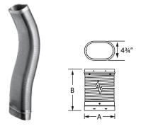
Use through damper and smoke shelf area. Built-in fittings. Use with DuraLiner ProMesh and ProFoil, where flex extends into clay liner, for zero clearance applications. Oval-to-Oval Flex pipe built from .016", 304 stainless steel, 4-ply construction.
