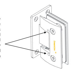
**4a.** Make sure the door glass is plumb and the edge of the hinge is installed flush with the glass edge. Center the hinge in the glass notch and tighten the faceplate screws (Figure 5a). Be careful not to scratch the finished surfaces of the hinge during installation.
