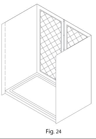
19. Mount the **Corner cover** (02) to the corner of the shower using the **Countersunk screws** ST4.2×30 (07).
