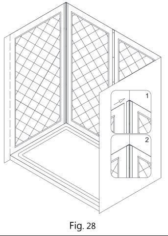
23. Once all panels are aligned, fasten tight the **Corner cover (02)** to secure the **Side panels (01)** and **Back panels (09).**
