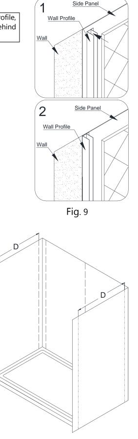
Measure the side walls of the shower from the 1" (one inch) line in the corner (from <u>Step. 1</u>) to the distance where you want Side panels (01) to end. The distance is "D".
