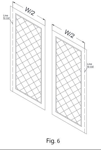
7. Place the **Back Panel (09)** onto a flat piece of plywood or particle board. Use a sharp industrial knife and a T-square to score along the marked side ends of the **Back panel** and continue scoring until you have fully cut through the panel.
