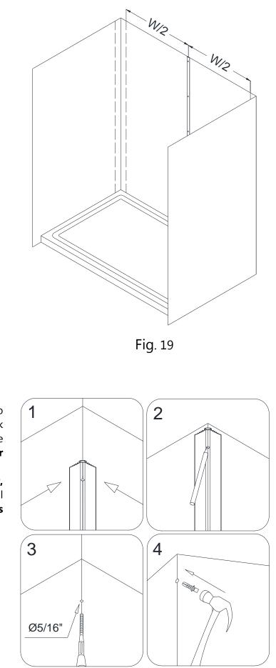
16. Attach the **Corner cover (02)** to the corner of the shower and mark the drilling holes through the predrilled holes in the **Corner cover**.
