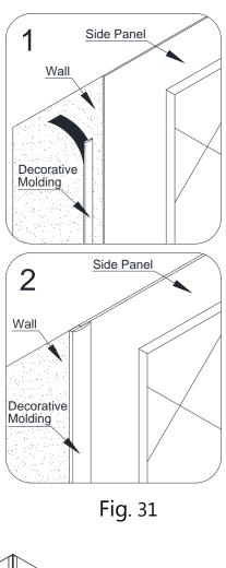
26. Apply caulk along the top edges of the **Side panels (01)** and the **Back panels (09).**
