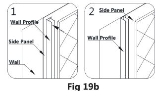
**20.** Apply adhesive to the entire back surface of the **Side Panel** (#01) for the opposite side wall installation. Use the same technique to apply pressure over the entire surface and make the top edge even with the
