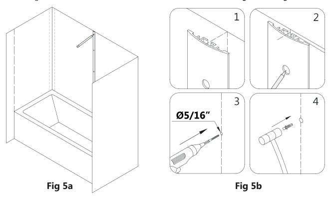
**6.** Place the **Corner Cover (#04)** to the corner of the wall and mark the drilling holes through the predrilled holes in the **Corner Cover (#04)**. Drill the holes using a **Ø5/16**" drill bit and insert the **Wall Anchors (#06)**. **(Fig 6a and Fig 6b)**
