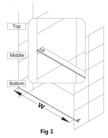
2. Subtract 3-3/8" from your finished opening (W) to determine the finished cut length for the Top and Bottom Guide Rails (#03). Cut the Top and Bottom Guide Rails (#03) to the finished cut length "D". Cut from the door end only, (which is the end farthest from the glass holder hole) and cut each rail to the same length from the same end. (Fig 2 and Fig 3)
