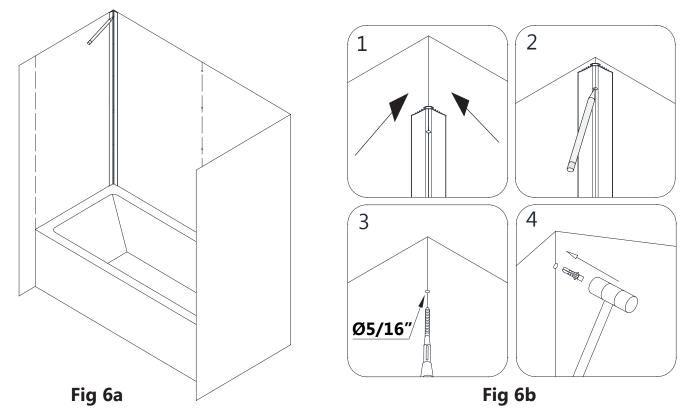
(If the finished overall width of the back wall= 59-1/2" from corner-to-corner, then it will not be necessary to trim the back panels. Proceed to **Step #9**).
