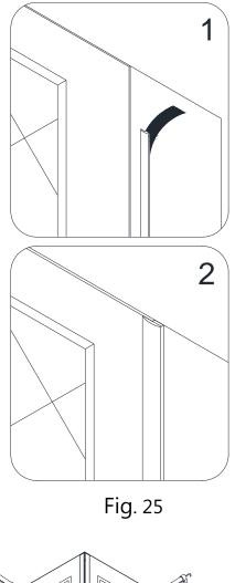
23. Apply caulk along the top edges of the Side panels (01) and the Back panels (09).Apply caulk along the connection of the bottom edges of the Side panels and bottom edges of the Back panels with the Shower base.
