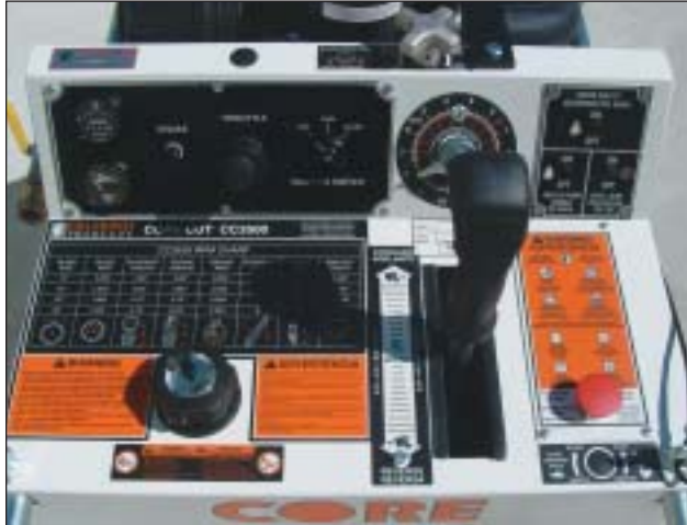
CC3500 Control Panel (shown with optional shaft tachometer and lowering speed metering valve)
