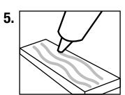
Use "Liquid Nail" or "PL Adhesive". Apply a generous amount to the back of the splash.
