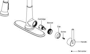
Many of these parts come preassembled. This exploded diagram is to assist in trouble shooting.
