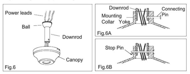
WARNING: Do not force connector pin through downrod. Use of force could cause damage to wires inside. Make sure the stop pin is properly engaged to prevent it from falling out.
