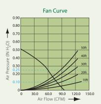
**Delta BreezSignature Ventilation Fan / LED Light Combo** Specifications
