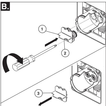
Insert adapter assembly (1) into valve body. Make sure the adapter assembly is correctly positioned and is pressed all the way down inside body. Secure adapter with the screw (2) provided in the adapter assembly. Remove the retainer (3) from the adapter.
