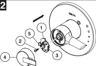
Secure temperature control knob (1) with screw (2). Hook (3) front of temperature control cover (4) onto knob (1) before engaging rear snap (5).
