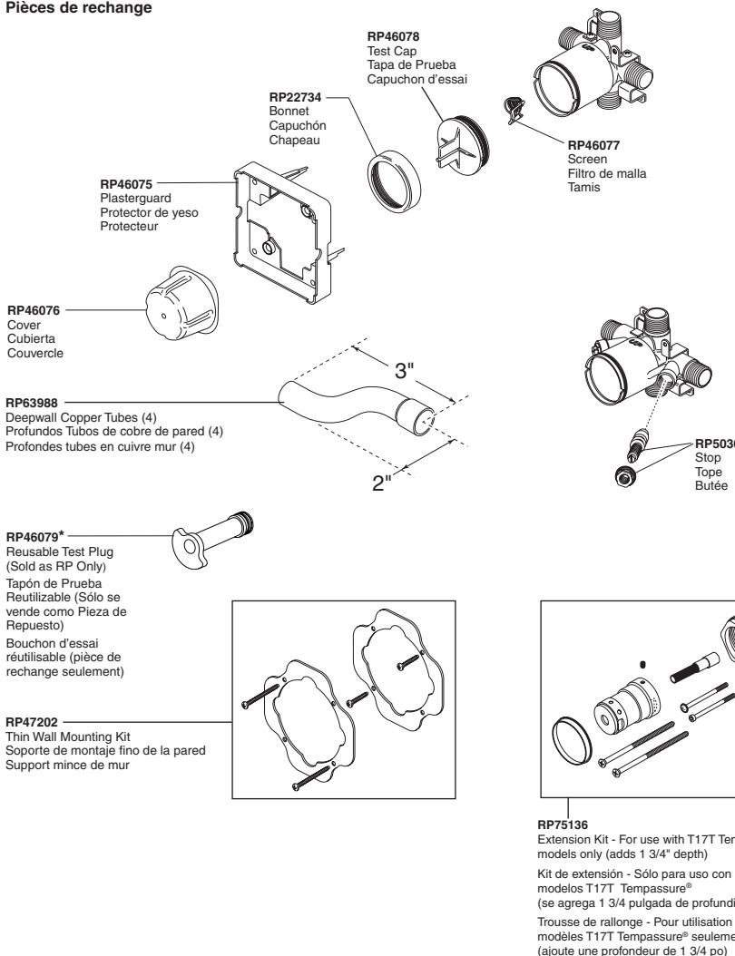
\*Used to plug one inlet side (Hot or Cold) to prevent cross flow when checking for leaks before the cartridge is installed. Insert into the inlet, place test cap and use the bonnet to secure in place.
