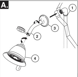
**FOR SHOWERHEAD INSTALLATION:** Connect top outlet (1) to shower arm (2) with proper fittings. To prevent damage to finish on shower arm, insert wall end of shower arm into shower flange (3) before screwing arm into riser connection. Thread showerhead (4) onto shower arm. Apply plumber tape to pipe threads on both ends. Do not overtighten showerhead.
