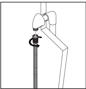
3. Attach the shower hose to the threaded supply outlet and proceed with the installation of the hand shower, following the manufacturers instructions.
