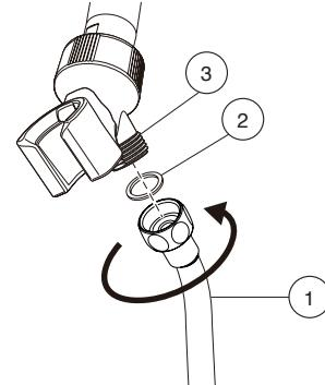
**A.** Ensure gasket (1) is inserted into the hose (2). Connect the hose to your designated water supply.
