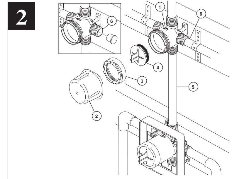
Consider the plumbing configuration and type and thickness of your finished wall before placing your stringer back plate (2).
