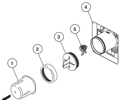
**Turn off water supplies.** Remove cover (1), bonnet nut (2) and test cap (3) from the body. If this is not a thin wall mounting, the entire plasterguard (4) may be removed. If screen (5) is in place, remove before installing cartridge.
