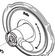
Place the temperature control knob (1) on volume handle and rotate to the mixed position (if required). DO NOT SECURE WITH SCREW. Turn on water supplies; let the water run until both hot and cold water is as hot/cold as possible. Place thermometer in a plastic tumbler, and hold the tumbler in the water stream. Record the temperature reading.
