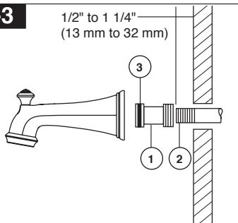
**Iron Pipe Installation****Installation of easy-on universal tub spout**
