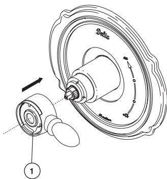
Install volume control handle (1) with lever to the right, then turn to the on position.
