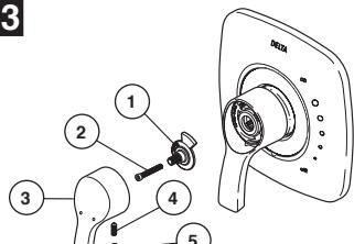
Secure temperature control knob (1) with screw (2). Install temperature control cover (3) and secure with set screw (4). Install button cover (5).
