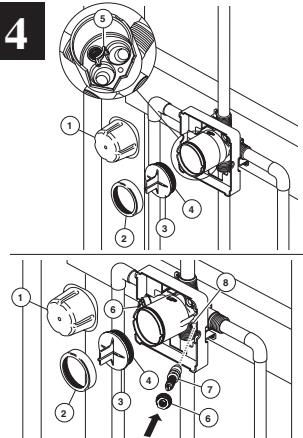
Connect top outlet (1) to shower pipe with proper fittings. Connect bottom outlet (2) to tub spout pipe with proper fittings. Pipe (3) between valve body and tub spout must be a minimum of 1/2" (13 mm) copper pipe or 1/2" (13 mm) iron pipe in a **straight** drop no less than 8" (203 mm) but no more than 18" (457 mm) long with only **one** iron pipe or copper 90 degree elbow to the tub spout nipple. **Do not use PEX tubing for tub spout drop.** Note: There is no tub outlet in high flow models.
