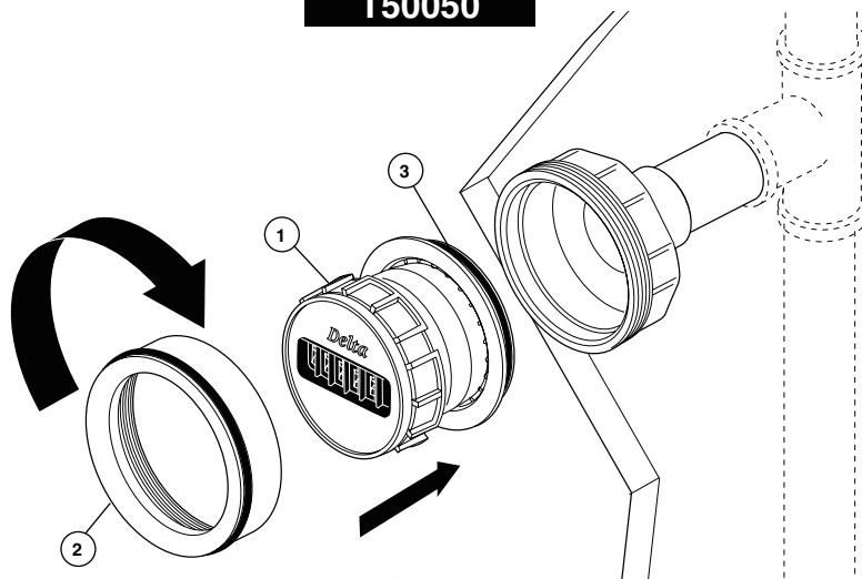
Remove plasterguard (1) and test plug (2) from the rough body.
