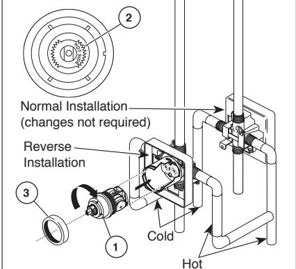
For back to back or reverse installations (hot on right and cold on left): Rotate cartridge (1) so the words "HOT SIDE" (2) appear on the right. Install the cartridge making sure that the key is fully engaged with the slot in the brass body (See step C). Slide bonnet nut (3) over the cartridge and thread onto the body. Hand tighten securely.
