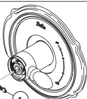
Secure temperature control knob (1) with screw (2). Snap on temperature control cover (3) with side snaps onto knob (1).
