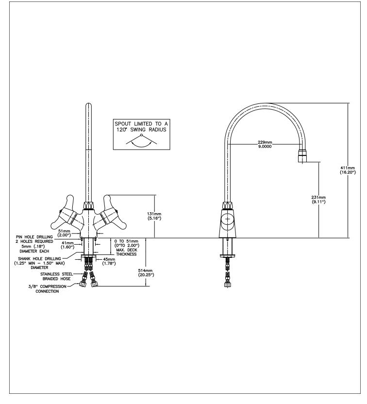
Delta reserves the right (1) to make changes to specifications and materials, and (2) to change or discontinue models, both without notice or obligation. Dimensions are for reference. Measurement may vary plus or minus 6mm(0.25"). Mounting locations are suggested only. Check with local codes for requirements in your area. This spec was produced July 18, 2013.
