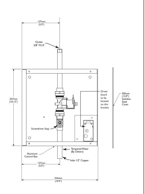
Note: For wallhung sink installations, sensor conduit rough-in should be directly under basin to minimize sensor cord exposure.
